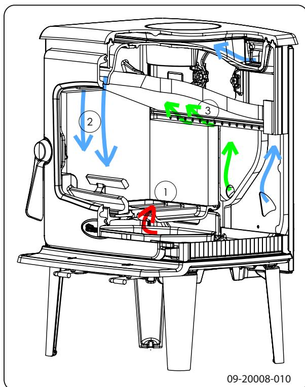
The primary air slide controls the air flow under the grille (1).
